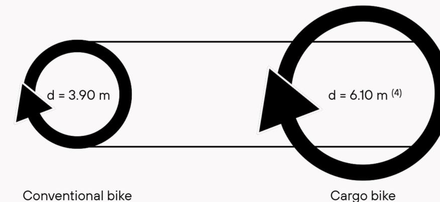
Fig. 28: Turning radii of different types of bicycles / © ARGUS. Data based on e-lastenrad.de.
